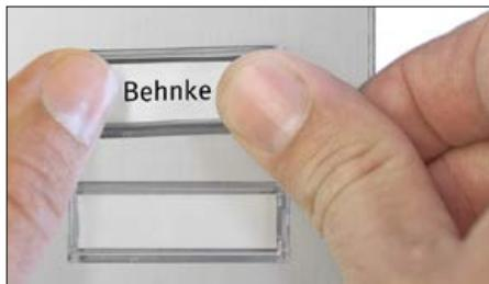
Press the labelling unit back into the intercom station – done.
